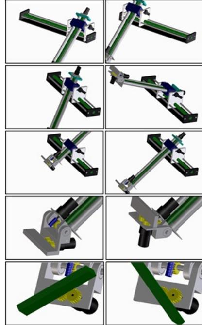
**Figure 3:** Demonstration of the working of the arm joints. In order from top to bottom: **1.** The panning joint. **2.** The elbow revolute joint. **3.** The retracting joint. **4.** The wrist pitch joint. **5.** The wrist roll joint
