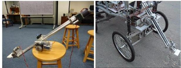
**Figure 1:** Sensor arm in lab (Left). Arm, controllers and stereo vision setup mounted on Marwa (Right).
