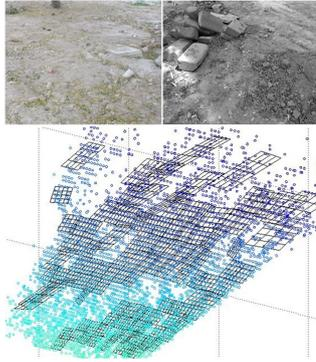
**Figure 6: top:** Example of an outdoor field used for Marwa’s experiments and a patch of uneven ground encountered during one of the scans. **bottom:** The corresponding point cloud. The point cloud has been overlaid by its piecewise planar representation, and rendered at a different angle for visual clarity.
