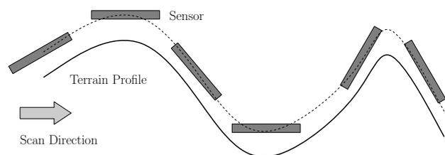
**Figure 5:** Cross sectional view of a single horizontal sweep of the metal detector.
