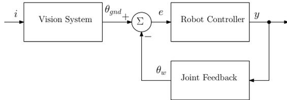
**Figure 2:** Block diagram for visual servoing of wrist pitch angle. Here  $i$  represents the stereo image pair,  $\theta_{gnd}$  is the angle of the ground normal and  $\theta_w$  is the wrist pitch angle. Similar controllers have been implemented for the rest of the arm joints.
