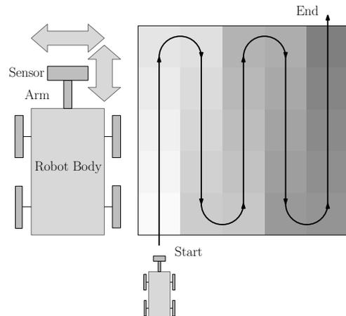
**Figure 4:** **left:** Possible scanning directions while Marwa is stationary. The sensor may be moved in forward or sideways direction. **right:** Coverage strategy of minefield adopted for Marwa. The path followed is indicated by the directed lines. A region is represented by a singly shaded area. Marwa scans a single region while remaining stationary and then moves to the next.
