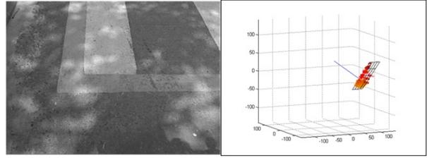
**Figure 10:** Sample image and corresponding point cloud with best fit plane and surface normal found by PCA
