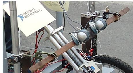
**Figure 7:** The stereo system mounted on Marwa.
