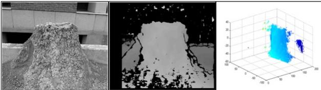
**Figure 9:** Snapshots of a scene, its disparity map and 3D point cloud as generated by our stereo system.
