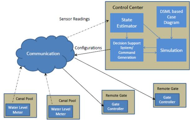
Figure 4. Smart water grids as cyber-physical systems [14].
