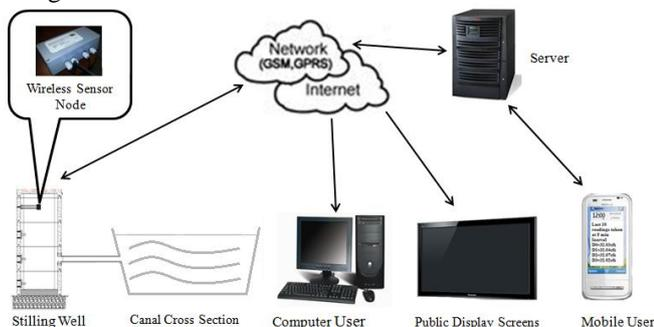
Figure. 4. Overview of a hydrometry network for canal flow measurement.
