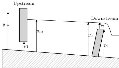
Fig. 5. Side-view sketch of Khaira Distributory Pool with undershot gate at upstream and 'hypothetical' overshot gate downstream (point of measurement). The value of  $p_2$  is always taken to be 0 to model an *always open* overshot gate.
