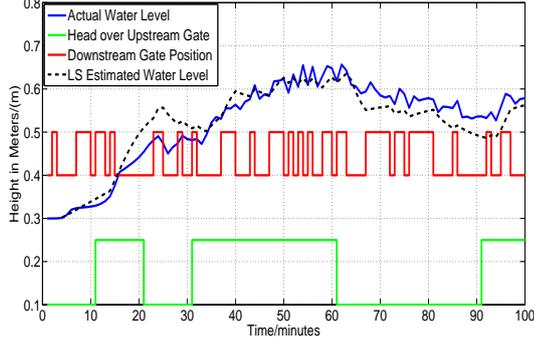
Fig. 4. Simulated & Estimated Response for Downstream Water Level.
