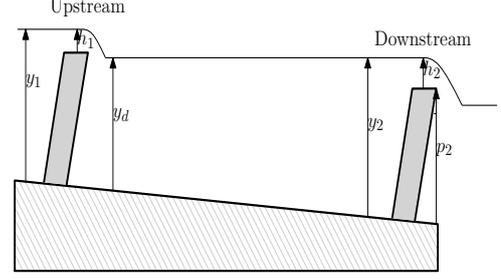
Fig. 2. Side-view sketch of a pool in open channel simulator with overshoot gates at upstream and downstream.
