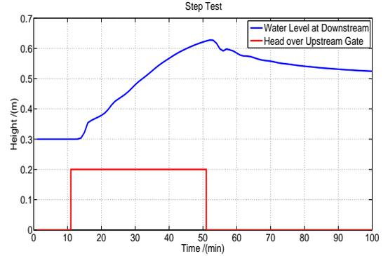
Fig. 3. Step Test for Open Channel.
