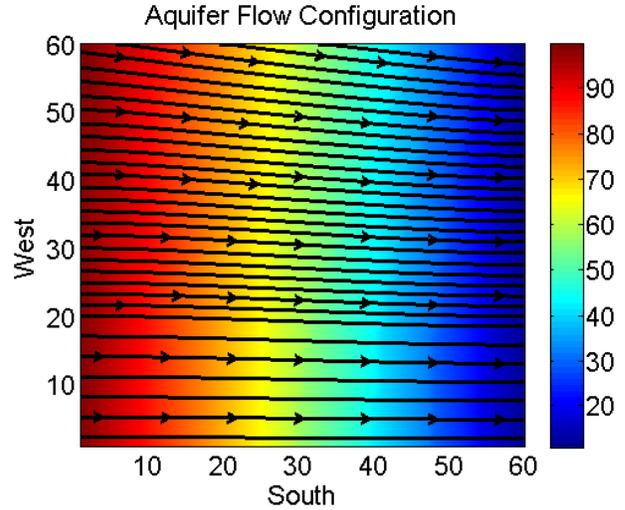
Fig. 6. Groundwater flow configuration in the two-dimensional  $60 \times 60$  grid. Arrows indicate the direction of flow groundwater. The color indicates the level of groundwater which is highest on the west side and lowest on the eastern end of the region.
