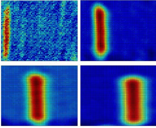
Fig. 9. 2D plot of the estimated contaminant level over 50 years in the groundwater. Estimates are obtained using Bayesian compressive sensing also making use of the additional knowledge about the aquifer flow configuration
