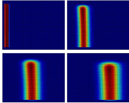
Fig. 7. Simulated 2D plot of the contaminant level over 50 years in the groundwater. The color here indicates the amount of contaminant in a cell in the groundwater.
