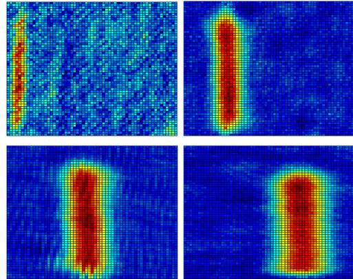
Fig. 8. 2D plot of the estimated contaminant level over 50 years in the groundwater. Estimates are obtained using Bayesian compressive sensing without using knowledge about the aquifer flow configuration
