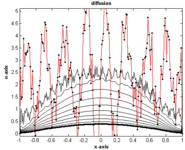
Fig. 4. Estimates of temperature state of the rod using Bayesian compressive sensing along with information about the model dynamics.
