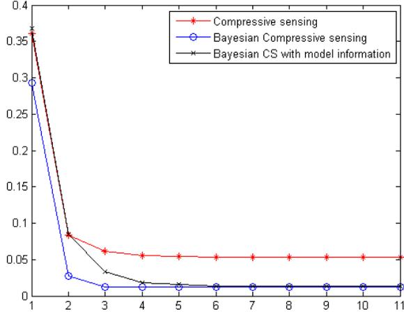
Fig. 5. Relative errors in the estimates of temperature states of the one dimensional rod. Estimates were obtained using  $l_1$  optimization, Bayesian Compressive sensing without model information and Bayesian CS with model information.
