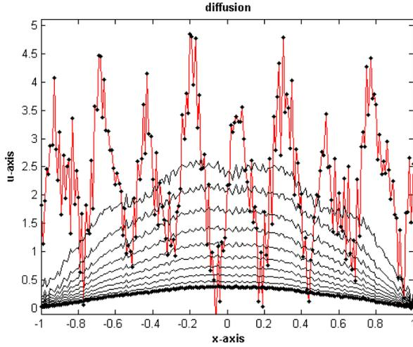
Fig. 2. (a) Estimates of temperature state of the rod using  $l_1$  norm minimization.
