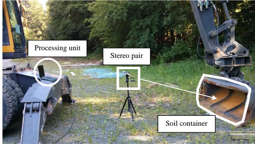
**Fig. 10.** Physical arrangement of real world setup.
