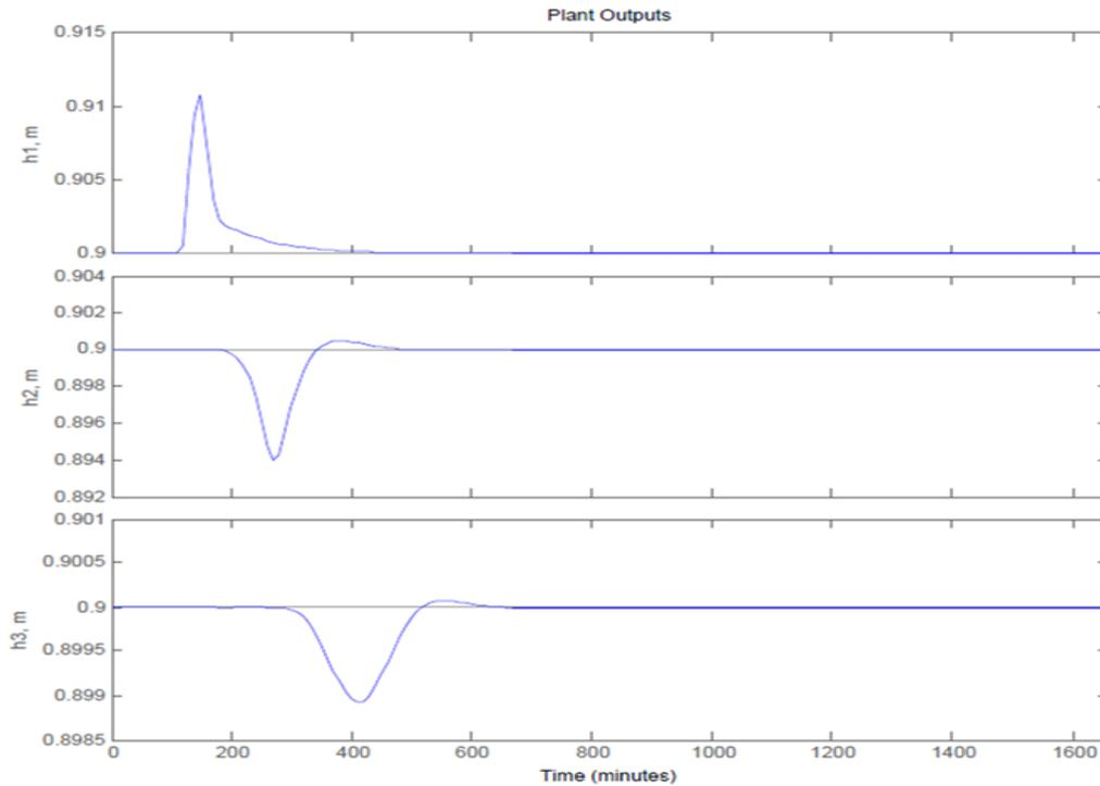
Figure 11: Water level in canal reaches is shown. Water level varies due to opening and closing of gates. Objective of MPC is to maintain at level at 0.9 meters.
