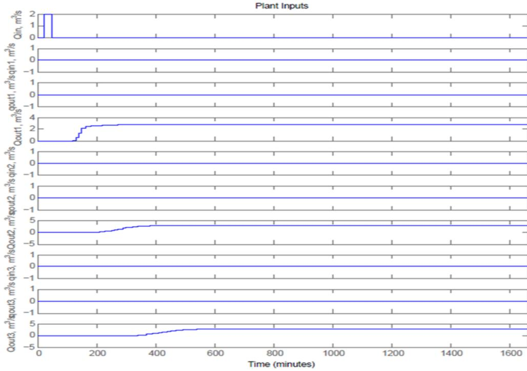
Figure 10: Inflows and Outflows in canal reaches by opening and closing of gates by MPC to maintain reference water levels. Input gate of canal reach 1 is opened for about 0.5 hour and there are no external disturbances.
