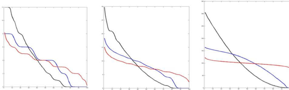
FIG. 3.2. Simplex distribution histograms for three sensor diameters: 0.16 units (left), 0.20 units (center) and 0.32 units (right). Each network is tested for three SimplexOwn protocols: Min (black), Median (Blue) and Random (Red). In all simulations, random assignment produces a better load balancing than other schemes (measured via distribution entropy).
