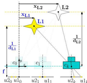
Fig. 1. The robot performing SLAM in a 2-D world with 1 beacon. Here,  $f$  is the focal length of the camera. Quantities highlighted in blue are known, whereas those in black are to be estimated.
