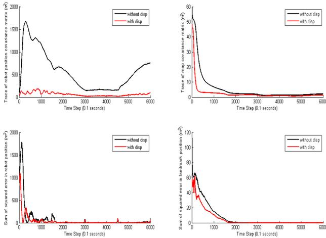
Fig. 4. Performance comparison between the conventional EKF and the generalized EKF presented in Section III. From top-left in counter clockwise order: 1) Trace of covariances for robot location, 2) Trace of covariances for landmark location, 3) SSD for robot location, 4) SSD for landmark location.
