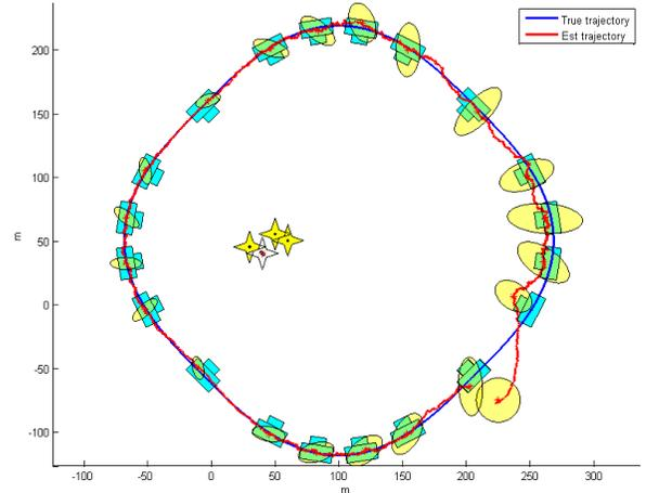
Fig. 3. A robot performing SLAM in 2-D. The cameras depict the true pose of the robot at selected time steps, equally distributed in time. The beacons are drawn in yellow whereas the estimated landmark is in white. The ellipses show the 95% confidence regions. An incorrect estimate with large uncertainty is provided.
