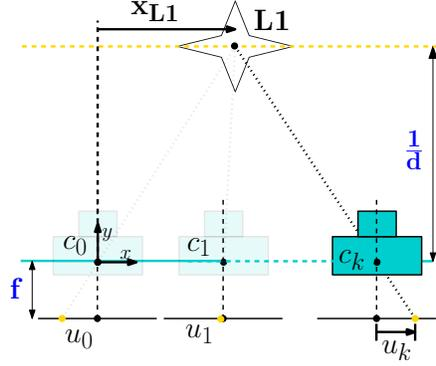
**Fig. 1.** The monobot performing SLAM with 1 landmark. The focal length of the camera is given by  $f$  and the inverse depth of the landmark is given by  $d$ .
