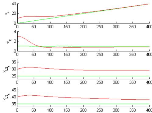
**Fig. 4.** State evolution with beaconization. After L2 is beaconized, its estimate levels off but the rest of the states continue to converge. A compromise on the convergence of L2 is the price we pay for being able to maintain observability.
