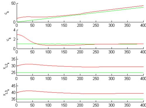
**Fig. 3.** State evolution without beaconization. The green trajectories represent the true state whereas the red trajectories represent the estimated states. The original beacon is obscured from sight at the 200th interval. From there onwards, the filter can be seen to diverge.
