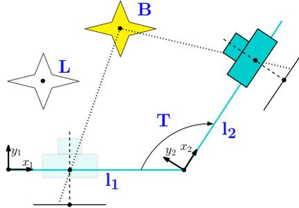
**Fig. 7.** Robot moving first along line  $l_1$  then along  $l_2$ . A landmark  $L$  and a beacon  $B$  are being measured. The transformation between the lines is given by  $T$
