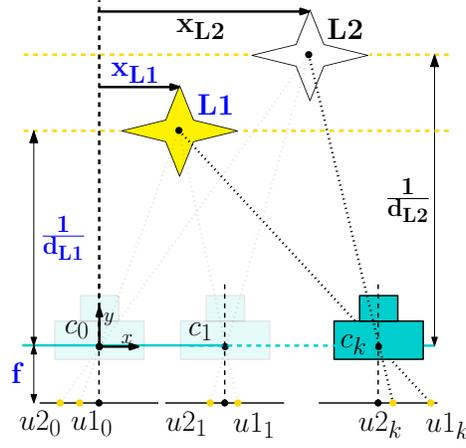
Fig. 5. The monobot performing SLAM in a 2D world with 1 beacon.
