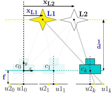
**Fig. 2.** The monobot performing SLAM with 1 unknown landmark and a beacon. Known quantities are written in blue.
