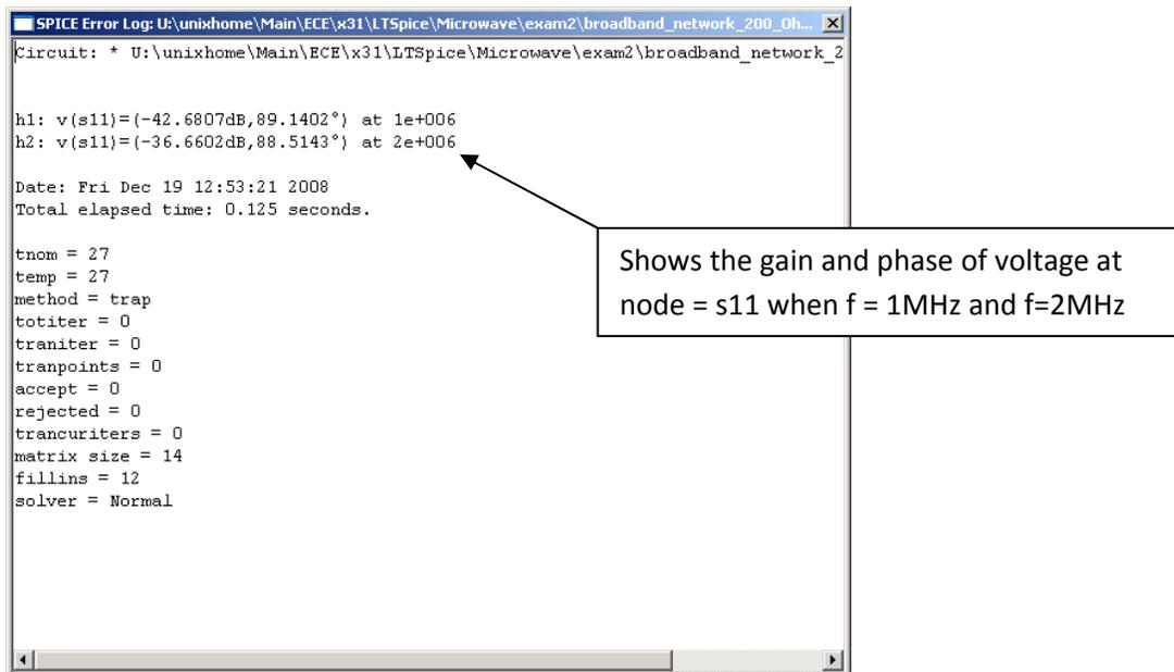
Figure 5.2.4 Gain and Phase shown in Error log from “View”
