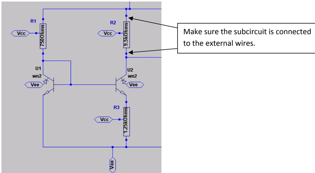
Figure 7.5 Subcircuits on a Main Schematic
