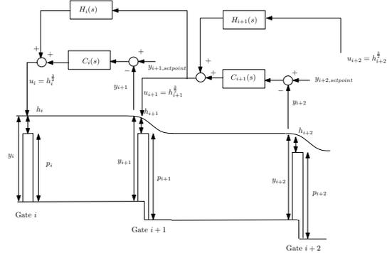
Fig. 9. Controller configuration in multiple pool
