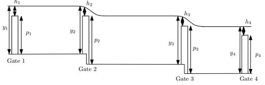
Fig. 4. Side view of pools and gates in an open channel.
