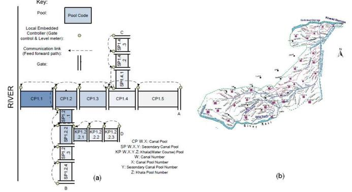
Fig. 12. (a) An example of irrigation network. (b) LCC canal network in Punjab, Pakistan. (Courtesy. Irrigation Department, Govt of Punjab)
