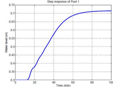
Fig. 5. Simulated step response of Pool 1.
