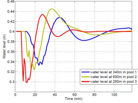
Fig. 10. Water level controlled in Pool 1,2 and 3.
