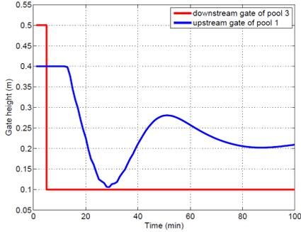
Fig. 11. Gate 1 behaviour during control action.
