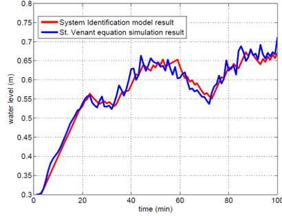
Fig. 7. Water level simulated using St. Venant equation and system identification model in Pool 1 at distance 340m
