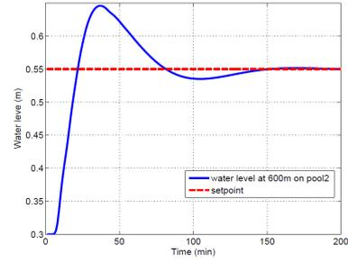
Fig. 8. Water level controlled on set point 0.55m in Pool 2
