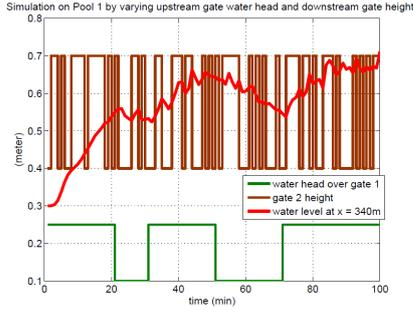
Fig. 6. Simulated water level in Pool 1 for a given scenerio.
