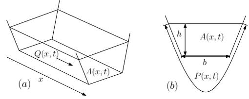
Fig. 2. (a) open channel flow along a longitudinal axis indexed by abscissa  $x$ . (b) cross-section of an open trapezoidal channel
