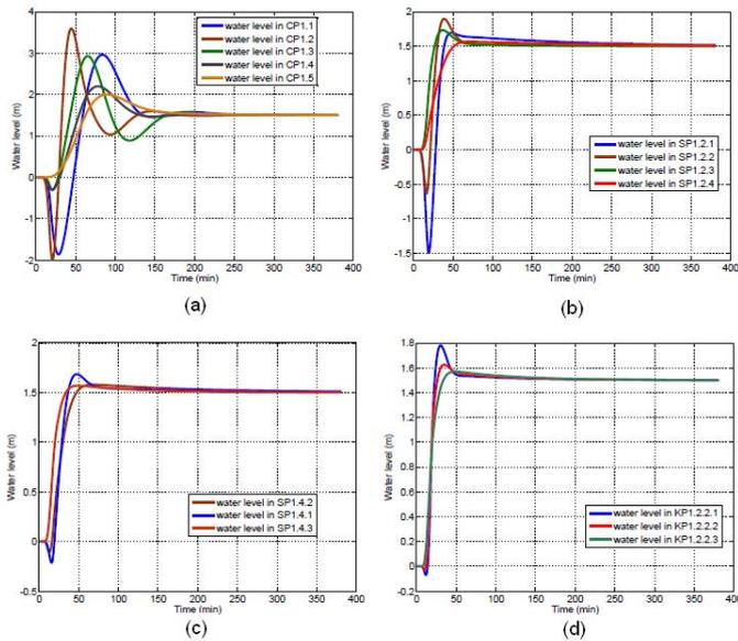
Fig. 13. (a) Water levels in main canal pools, (b) Water levels in secondary canal pools emerging from CP1.2, (c) Water levels in secondary canal pools emerging from CP1.2, (d) Water levels in khala pools emerging from SP1.2.2.
