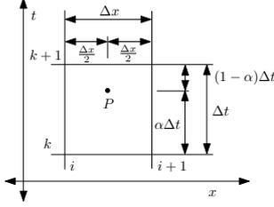
Fig. 3. Grid point for the Preissmann scheme
