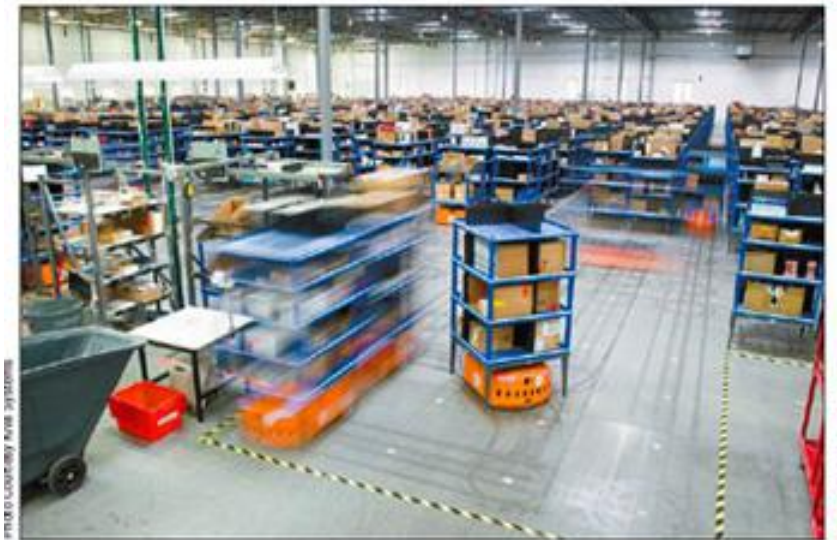
Robots zoom around a warehouse. The robots, which can carry either 1,000 pounds or 3,000 pounds, travel on tracks and are manufactured by Kiva Systems of Woburn, Mass.
