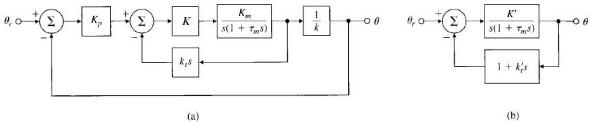
1. Find values for  $K'$  and  $k'_t$  so that the system of figure (b) has the same transfer function as the system of figure (a).
