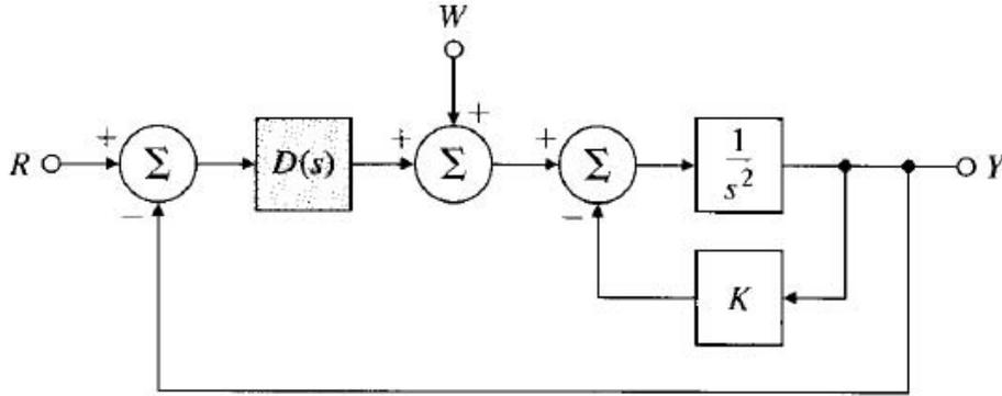
1. What condition must  $D(s)$  satisfy so that the system can track a ramp reference input with constant steady-state error?
