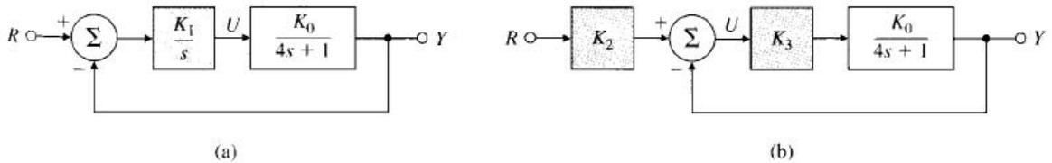
1. Determine values for  $K_1$ ,  $K_2$  and  $K_3$  so that both systems exhibit zero steady-state error to step inputs (that is both are type 1) and whose static velocity error constant  $K_v = 1$  when  $K_0 = 1$ .
