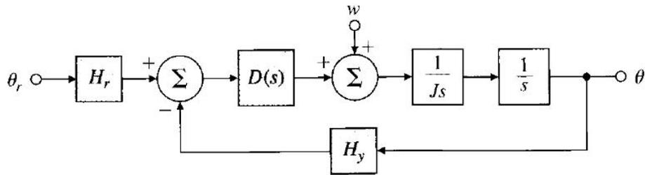
1. Use proportional control, P with  $D(s) = k_p$ , and give the range of values for  $k_p$  for which the system will be stable.
