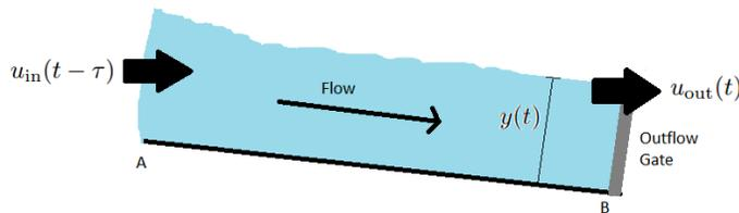
Figure 1: Irrigation channel model for Problem 3.
