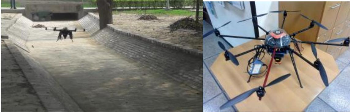
**Figure 3.** An octocopter during canal inspection operation over a channel in LUMS campus (Left). Close-up of the flying machine being configured in lab (Right).
