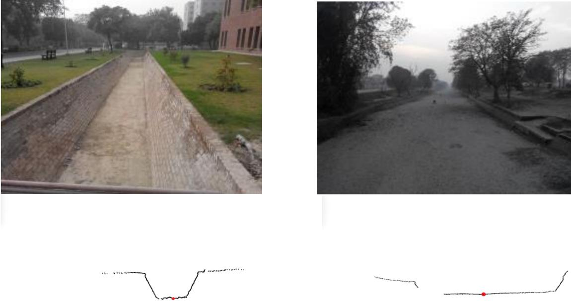
**Figure 8.** Center point calculation from laser scans obtained over two test scenarios. The algorithm output is marked by a red dot. A small lined channel with symmetric geometry and good data fidelity (Left). A large channel with corrupted measurements and less symmetry.
