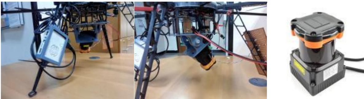
**Figure 4.** Odroid single board computer mounted on one aerial machine leg (Left). Laser scanner mounted underneath robot using a 3D printed mount (Center). Also, seen in pictures is a custom-built voltage regulator attached to another leg. Hokuyo Laser scanner used in this work (Right). All these accessories count towards the external payload of the robot which must be under 2500g as per specification of the UAV.
