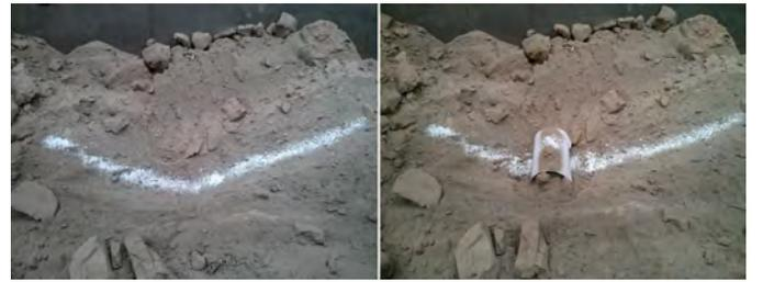
Fig. 12. Two states of the channel model for volume experiment: (a) Baseline (left); (b) Silted (right).
