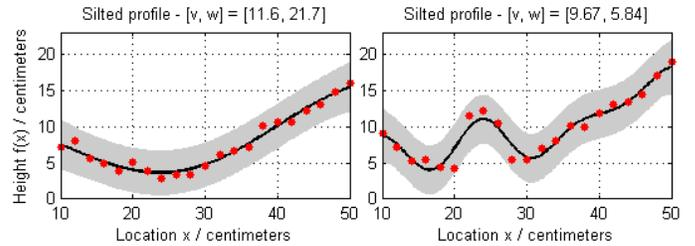
Fig. 13. Corresponding surfaces of the two states of the channel model - Baseline (left) and Silted (right) (See Fig.12). For both,  $\sigma_r^2 = 1.44 \text{cm}^2$  and  $\sigma_p^2 = 0 \text{cm}^2$ .
