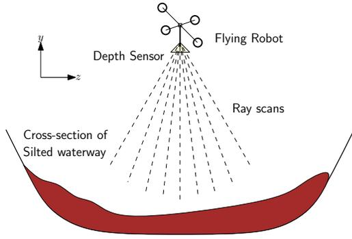
Fig. 3. Cross-sectional view of a silted canal bed profiled by a flying robot.
