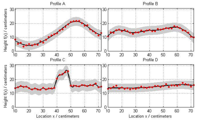
Fig. 11. GP Regression results with optimal parameters of the corresponding profiles (See Fig. 10). Note that, we took  $\sigma_r^2 = 1.44 \text{cm}^2$  and  $\sigma_p^2 = 0$ .
