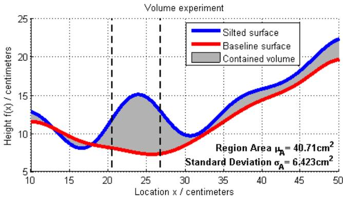
Fig. 14. Plots depicting one-dimensional view of the silt volume estimation experiment. The hump enclosed by the dashed lines represents the approximated surface of the cylindrical object used (See Fig. 12). The difference in surfaces outside this region is because of noise in sensor readings.
