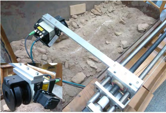
Fig. 9. Hardware assembly of scaled lab model depicting a scene of a silted canal bed, with a scanner maneuvering above it along length axis. Close-up of LMS151 scanner shown in bottom-left.
