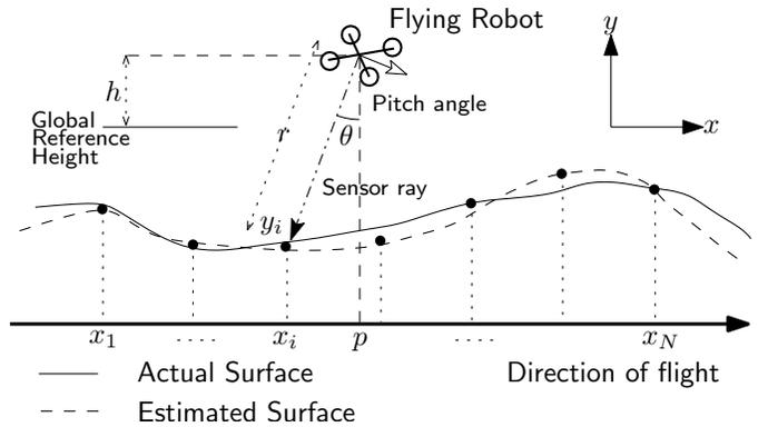
Fig. 2. Side view of a silted canal bed being profiled by a flying robot.
